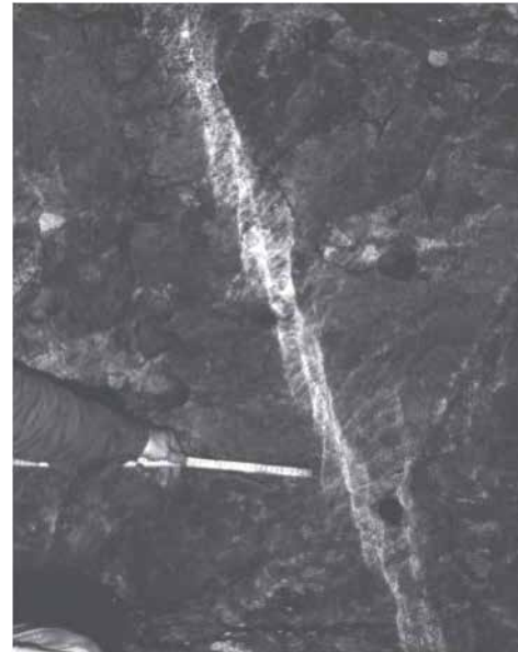
Figure 68: Ruler pointing at shear rupture, known as Rupture No. 18 (Ortlepp, 1997)
