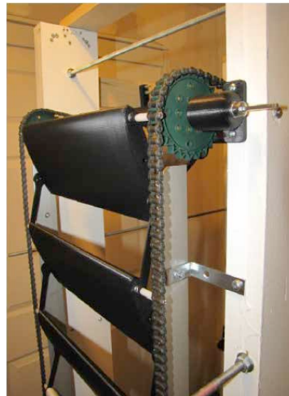
Figure 114: An air flow regulator that provides resistance by recovering air flow energy by using moving blading to drive an electrical generator
