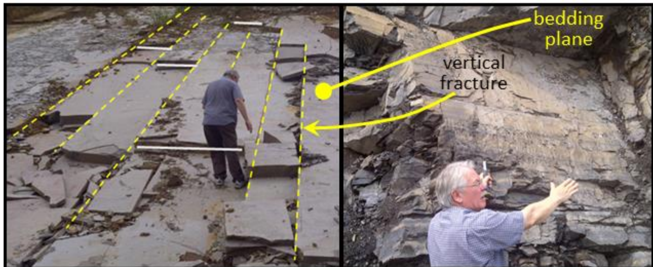
Figure 1: Joint Sets in Outcrops of the Oil Source Rock, Central Sumatra Basin.
