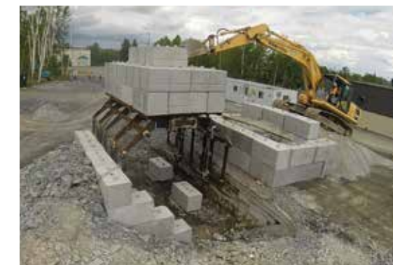
Canopy strength test with 75 tonne load simulation
