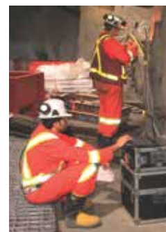
Ramin Saleh and Derek Zwaan, University of Toronto, using a Scintrex gPhoneX Gravimeter and installing geophones on rockbolts. Photo courtesy of Chris Pritchard
