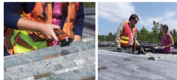
Physical properties logging of drill core at the Victoria Project site of KGHM. Courtesy of Melissa Pecman
